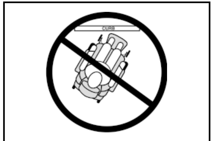
Figure 3. Incorrect Curb Approach
